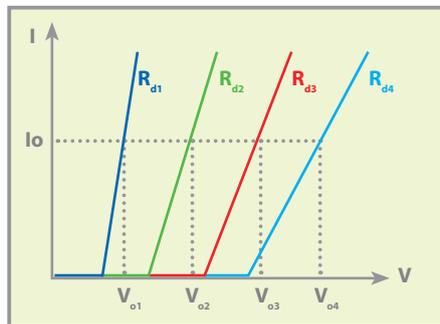
Figure 2 - Simulate different number of LEDs
