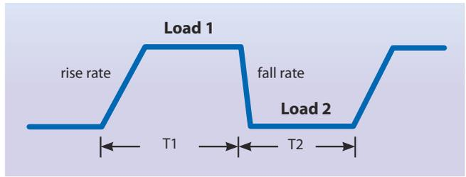
The programmable slew rate makes the simulation of transient load change demanded by real life applications possible. The 6310A internal waveform generator is capable of producing a maximum slew rate at 10A/μs, and dynamic cycling up to 20kHz. Its dedicated remote load sense and control circuit guarantee minimum waveform distortion during continuous load changes.
