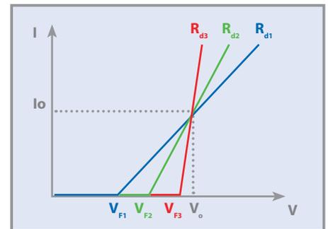
Figure 3 - Simulate different characteristic of LEDs
